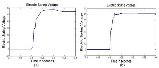
Figure 9. Electric Spring voltage during (a) under voltage conditions (b) over voltage condition
