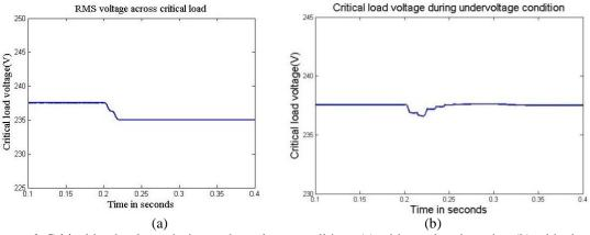
Figure 6. Critical load voltage during under voltage conditions (a) without electric spring (b) with electric spring
