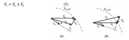
Figure 2. Phasor diagram of Electric Spring (a) inductive mode (b) capacitive mode
