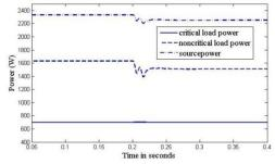
Figure 10. Measured source power, noncritical load power and critical load power during over voltage conditions
