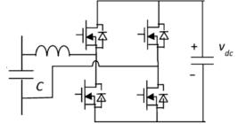
Figure 3. Full H bridge inverter employed in the scheme
