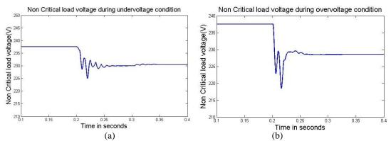
Figure 8. Noncritical load voltage during (a) under voltage conditions (b) over voltage conditions
