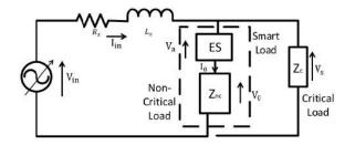
Figure 1. Overview of electric spring in series with noncritical load
